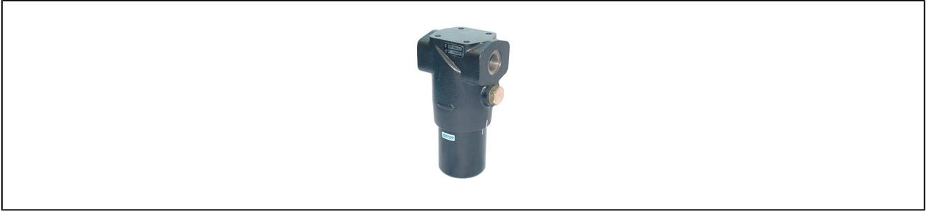
description pressure filter series HPM filter material cellulose fibre; -20...+95°C; max. operating pressure 420bar; max. differential pressure 20bar; bypass valve; opening pressure 6bar
