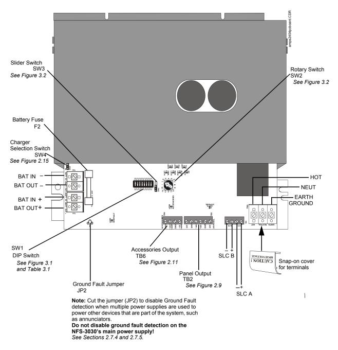
Figure 1.1 The AMPS-24 Board Layout
