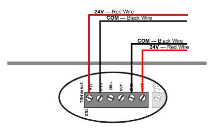
Figure 2.9 Connecting to the Panel Output TB2
