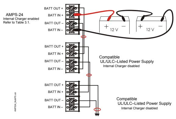
Figure 2.19 Connecting Multiple Power Supplies
