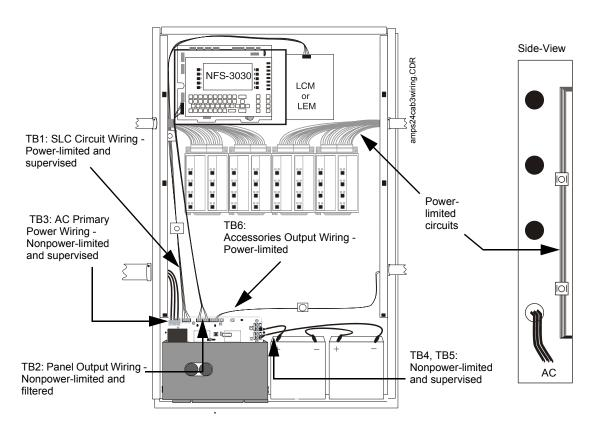
Figure 2.6 CAB-4 Series Cabinet: Power-limited Wiring Example
