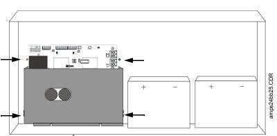
Fasten the power supply to the backbox with (4) self-threading screws at the indicated positions.
