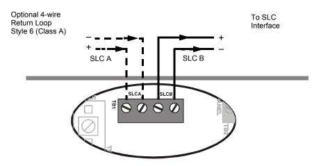
Figure 2.10 Connecting to the SLC Interface TB1
