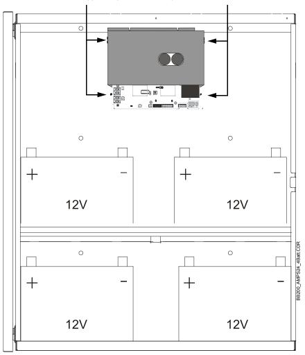
Fasten the AMPS-24 chassis to the backbox using the four supplied keps nuts at these positions.
