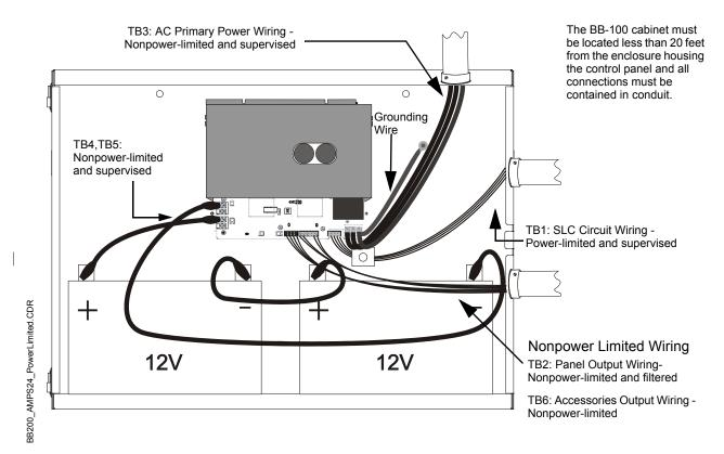
Figure 2.7 BB-100 Cabinet: Power-limited Wiring Example with Two Battery Wiring
