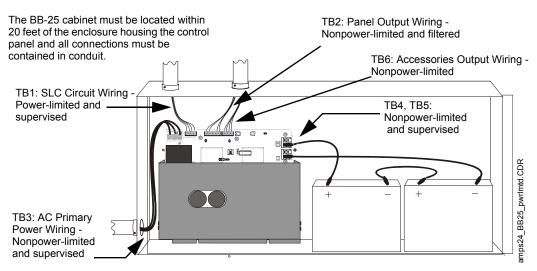
Figure 2.5 BB-25 Cabinet: Power-limited Wiring Example, with Two Battery Wiring
