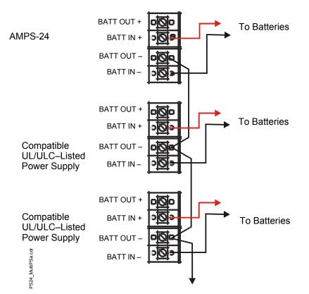
Figure 2.18 Connecting Multiple Power Supplies with Common Bond Wire
