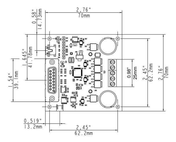
FIGURE 18. SBL13xx top view and dimensions
