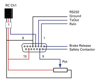
FIGURE 14. Factory default pins assignment
