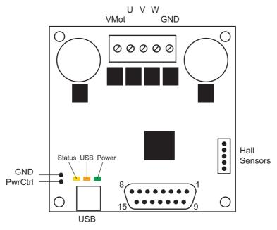
FIGURE 8. Controller Layout
