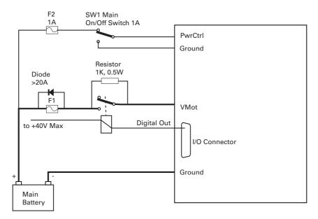
FIGURE 10. Contactor wiring diagram
