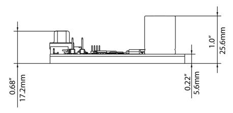
FIGURE 17. SBL13xx front view and dimensions
